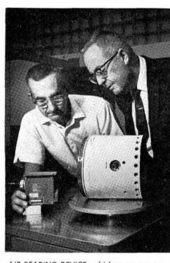
AIR BEARING DEVICE, which measures moment of inertia almost independent of the test object's weight, is positioned by designer C. E. Miller (left) while his supervisor, R. N. Browne (7214), follows the operation.
